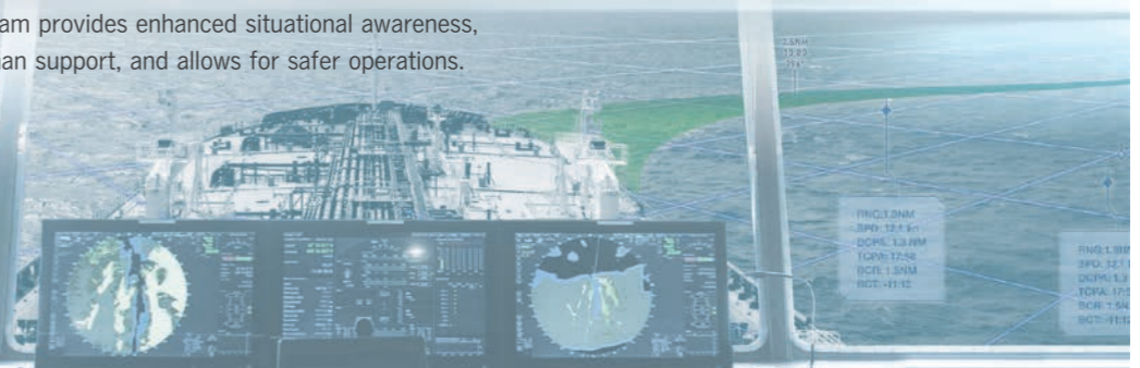
Display image of the AR Navigation system. Azimuth, AIS, Own ship position, ship speed, and other information such as the route and waypoints are superimposed over the live video imagery.
