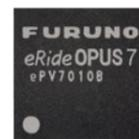
GPS (GNSS) Receiver Chip & Module
