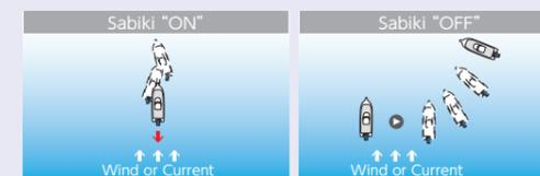
With the SABI mode turned on, the direction can be kept just by adjusting the throttle.
