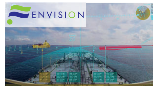
Display image of the AR Navigation system. Azimuth, AIS, own ship position, ship speed, and other information such as the route and waypoints are superimposed over the live video imagery.
