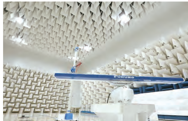
EMC testing of a radar antenna
