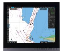
ECDIS (Electronic Chart Display and Information System)
