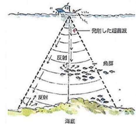
Principle of ultrasonic fish detection
